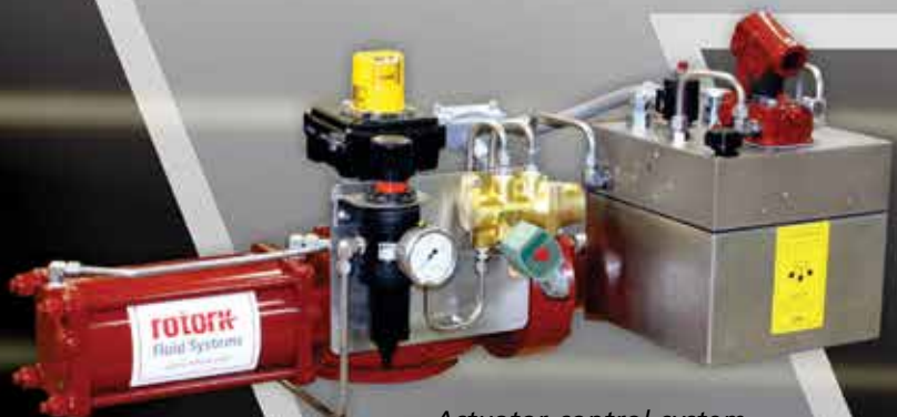
Actuator control system for pump control valves
