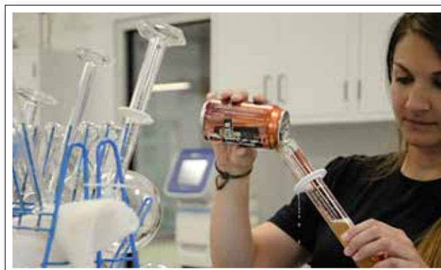
Avery Brewing’s lab tests beers 20 times from grain to glass. Microbiologists and chemists use lab equipment to determine the cell count, cell size, viability, and vitality of the brewer’s yeast and measure the color, bitterness, and diacetyl of beer to maintain high quality and consistency. Photo courtesy of Avery Brewing Co.
