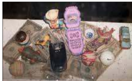
Nondispersibles found in the Kennebec Sanitary treatment District (Waterville, Maine) system during a facility inspection. Photo courtesy of Aubrey Strause, Verdant Water PLLC (Scarborough, Maine) owner.
