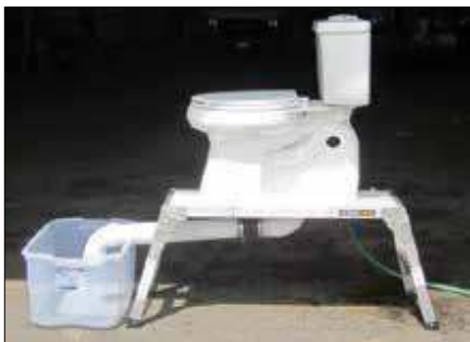
Robert Villée, Plainfield Area Regional Sewerage Authority (Middlesex, N.J.) executive director, worked with authority staff to test flushable-product claims using this system. Photo courtesy of Villée.
