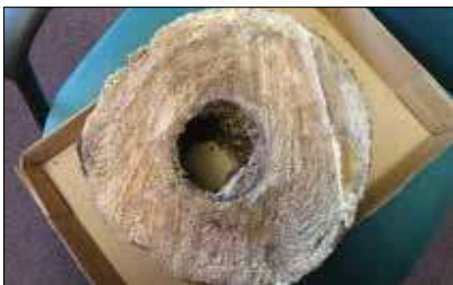
Interesting note: wooden water mains uncovered during an excavation.
